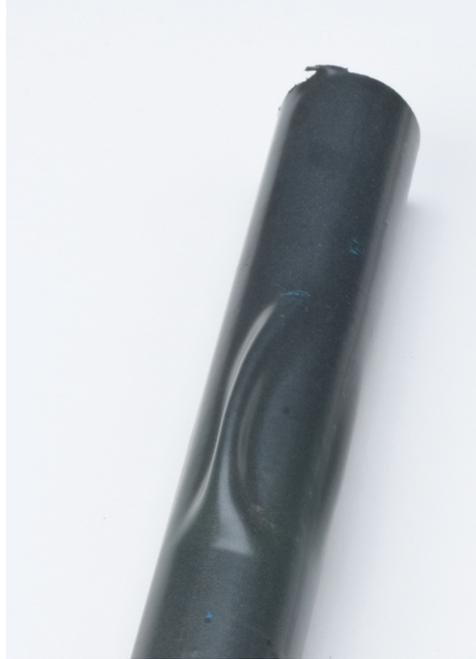
*Photo Caption: The PVC coating has blistered due to poor adhesion of the coating to the substrate.*
