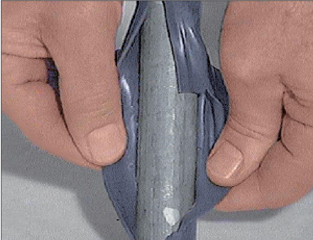
**Figure Above:** shows a PVC coated conduit specimen where the coating adhesion has failed. This conduit sample was exposed for approximately two days in the Hot Water Immersion Test. Once the cuts are made, the PVC coating is easily removed by pulling the coating by hand. The PVC coating is torn to expose the galvanized steel conduit in the photograph.
