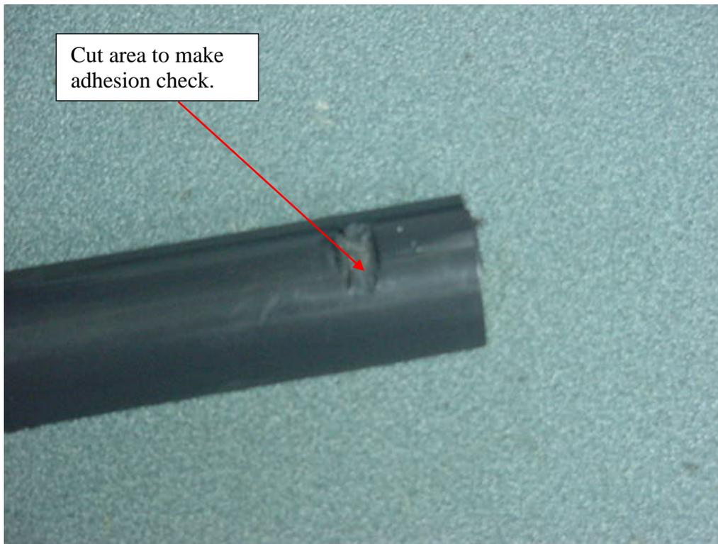
**Figure Above:** PVC Coated Conduit Specimen with Acceptable Adhesion.
